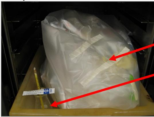
Ampule in center of autoclave waste bag.
