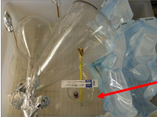
Beaker containing thermometer and ampule with strip on top, inside bin with glassware.
