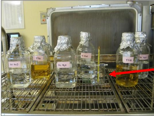
Beaker containing thermometer with strip on top, amongst bottles of TSB (2) and DI water (4).
