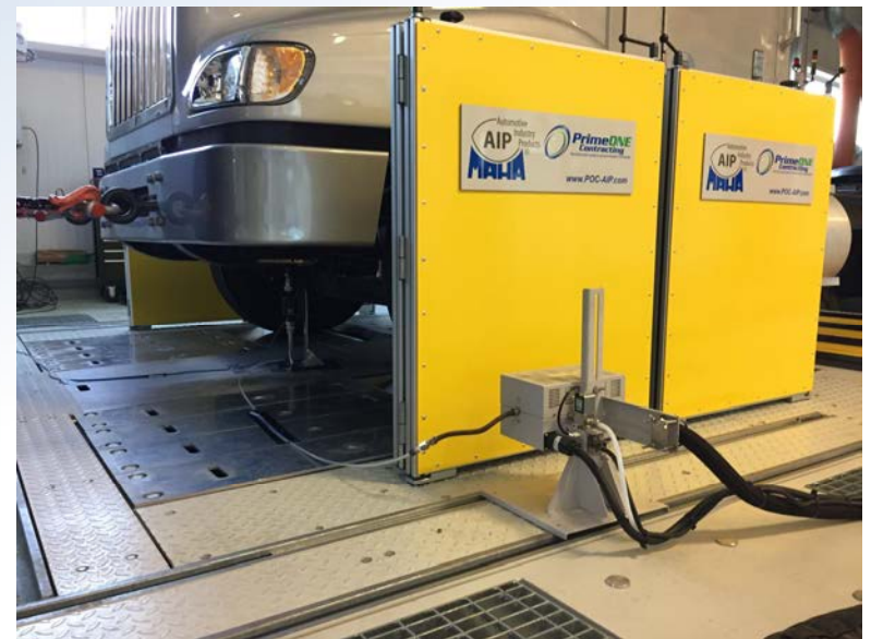
NVFEL testing used to estimate crankcase emissions for 2010+ HD trucks
