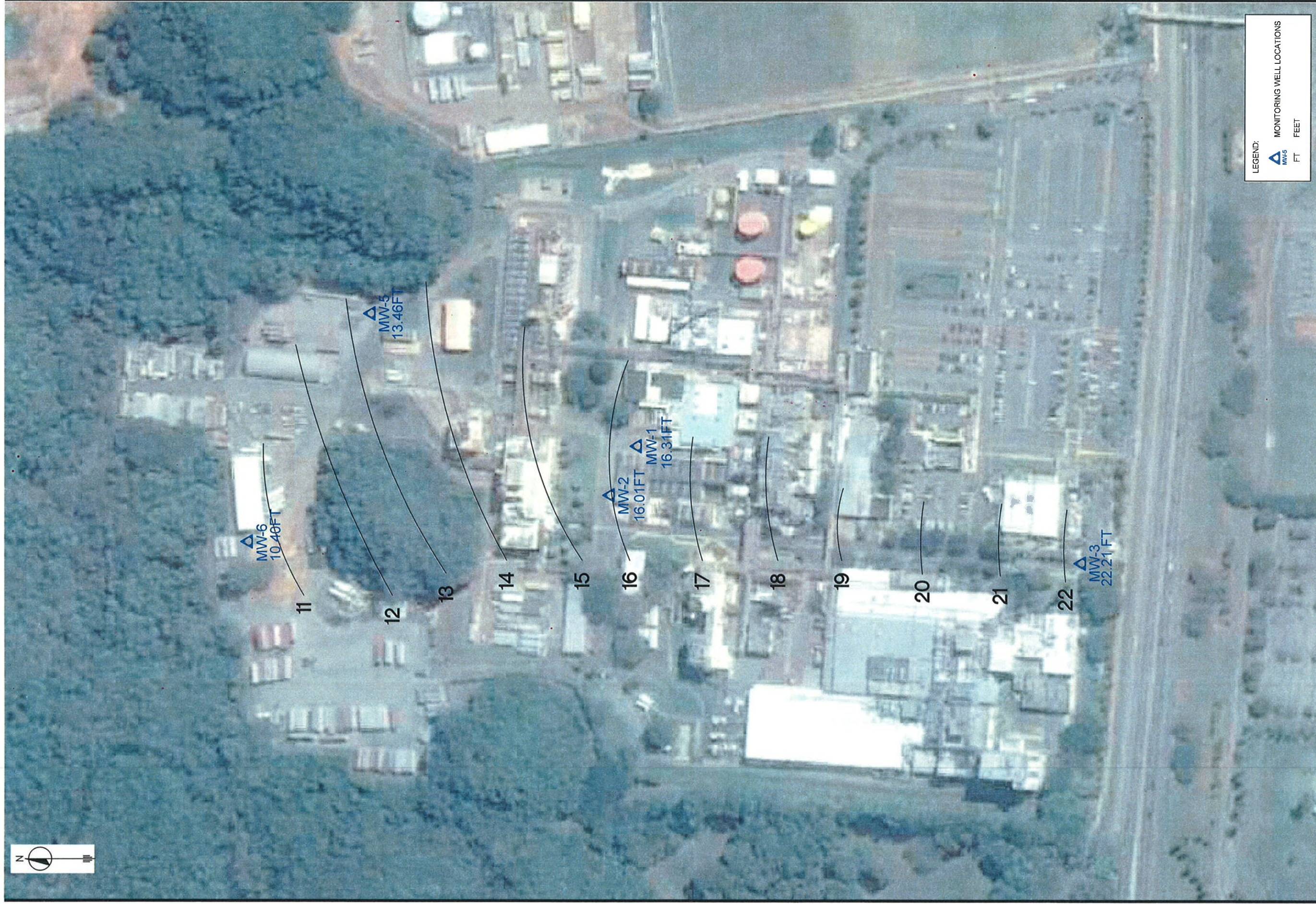
FIGURE 3 - GROUNDWATER CONTOUR MAP - JULY 2018 PFIZER PHARMACEUTICALS, LLC BARCELONETA, PUERTO RICO
