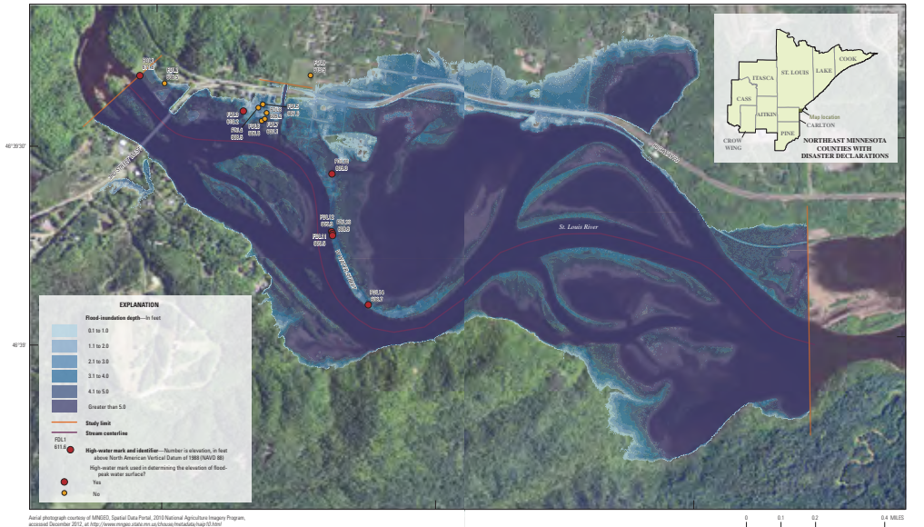
► Figure 8. Approximate extent and depth of flood peak inundation at the Fond du Lac Neighborhood in Duluth Source: Czuba et al., 2012
