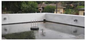
Photo 29.1 Example of flood test at the Denver Botanic Garden green roof. Photo courtesy Mark Fusco
