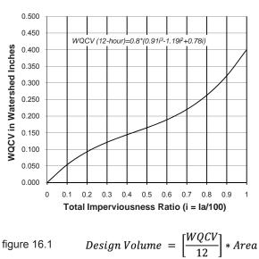
Water Quality Capture Volume (WQCV) for a BMP with a 12 Hour Drain Time
