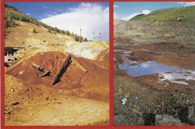
Top: The eerie effects of windblown tailings near the former Mary Murphy Mine and Mill in Colorado. Bottom Left: Tailings and the remains of historic mine workings exhibit the characteristic reddish-brown color of iron oxide leaching. Bottom Right: Blocked by mine waste dumped in the stream channel, the flow in French Creek was reduced to ponding near the former Wellington-Oro Mine near Breckenridge, Colorado.
