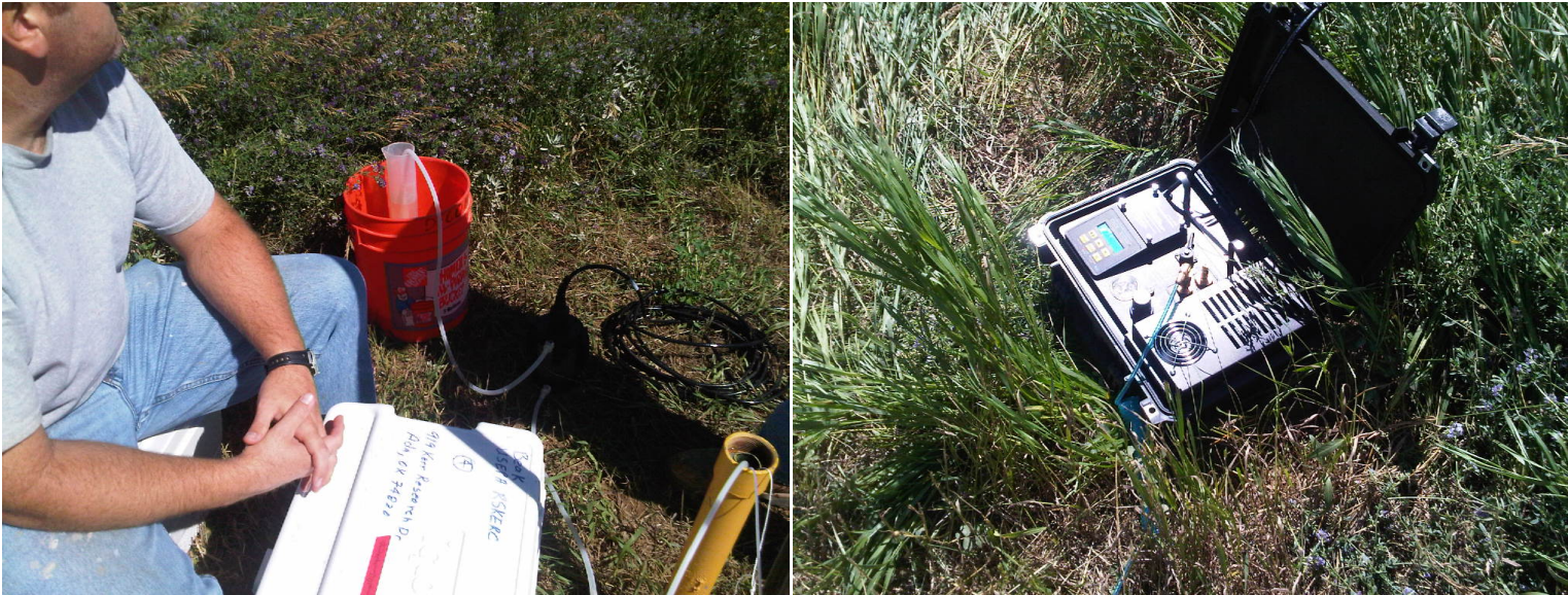
Figure 11. North Dakota Water Commission well sampling and bladder pump controller.
