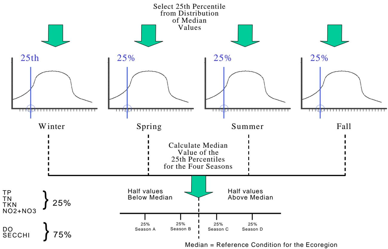
**Figure 4b. Illustration of reference condition calculation.**
