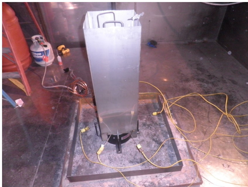
Figure 3-7. Photograph of Burn Chamber for High-Temperature Conditions.
