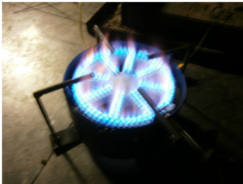
Figure 3-6. Photograph of Propane-Fired Ring Burner.
