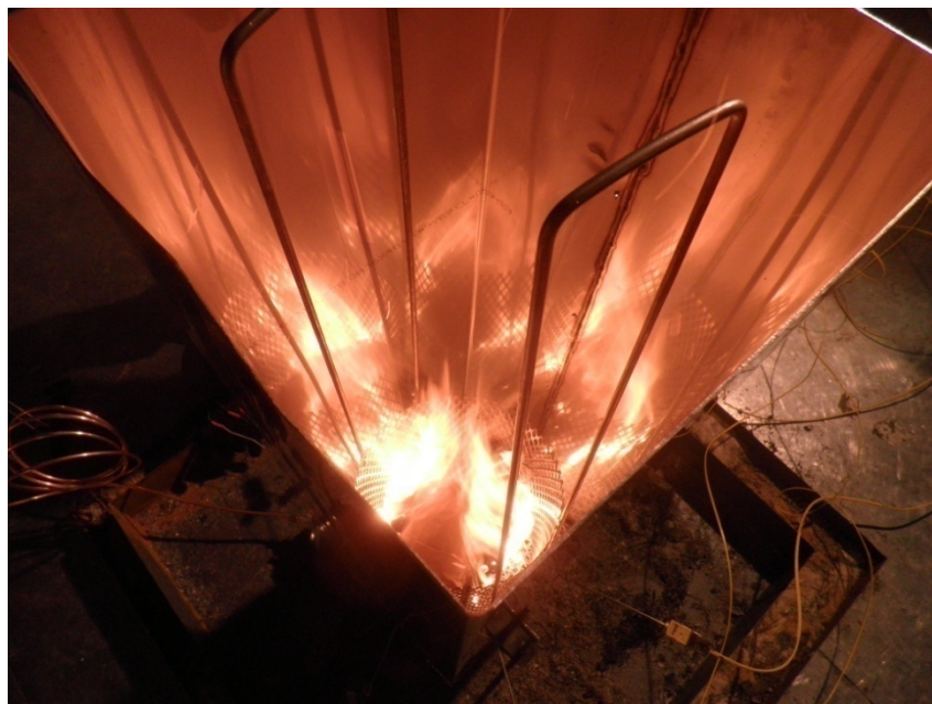
Figure 3-9. Photograph of Duff Combustion — High Temperature Scoping Test.
