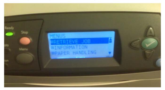
Press the **Menu** button on the printer. Use the arrow keys to select the option **RETRIEVE JOB**. Press the **green button with a white checkmark**.
