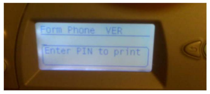
Press the UP and/or DOWN **arrow keys** to enter a digit. Press the LEFT and/or RIGHT **arrow keys** to move to the next position. After entering the 4 digits, press the **green button**.
