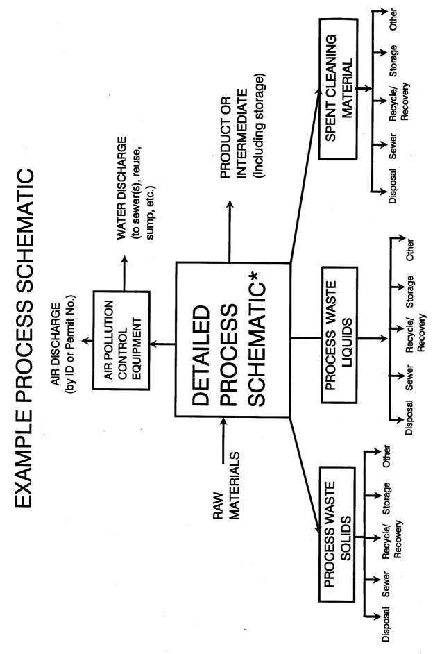
\* The process schematic should be detailed and may require may boxes to adequately depict. Material quantities and process units need to be identified.
