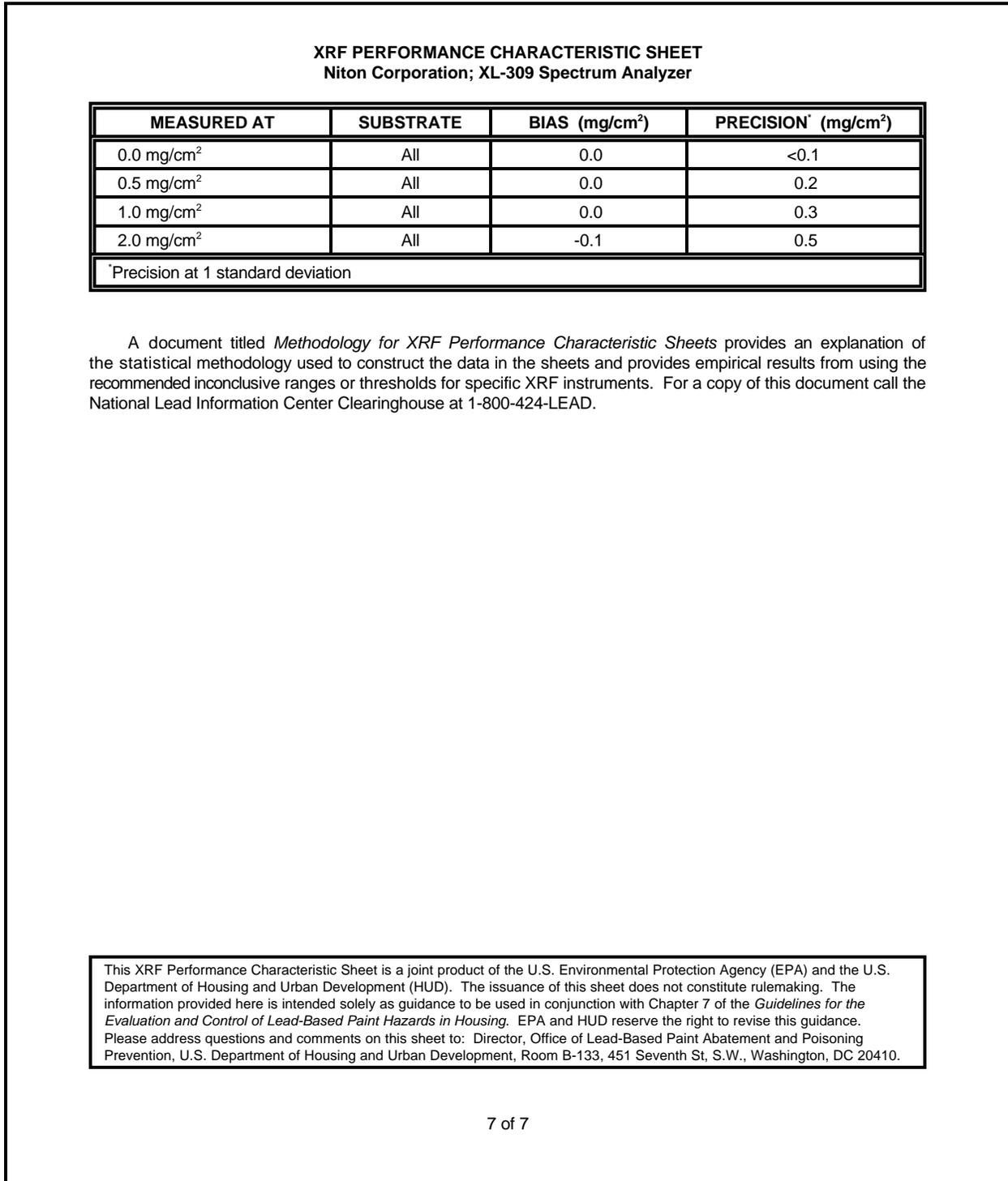
Figure D-8 continued. XRF Performance Characteristic Sheet for the Niton XL-309 Spectrum Analyzer.
