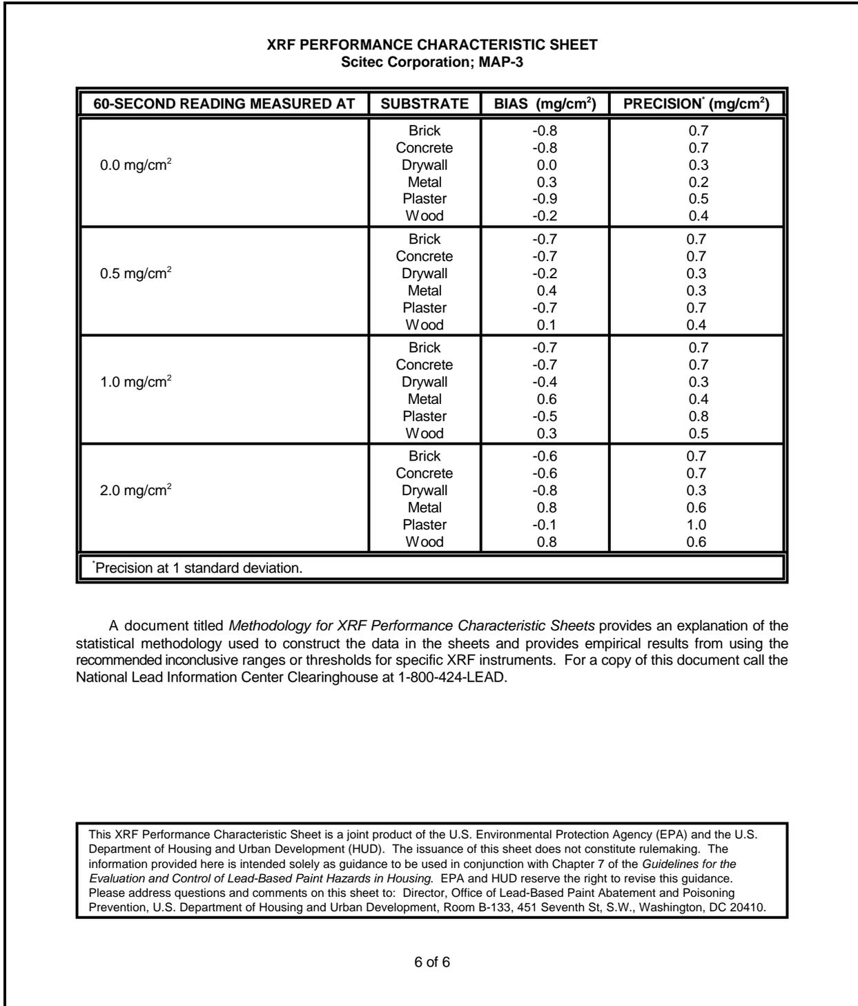
Figure D-3 continued. XRF Performance Characteristic Sheet for the Scitec Corporation MAP-3.
