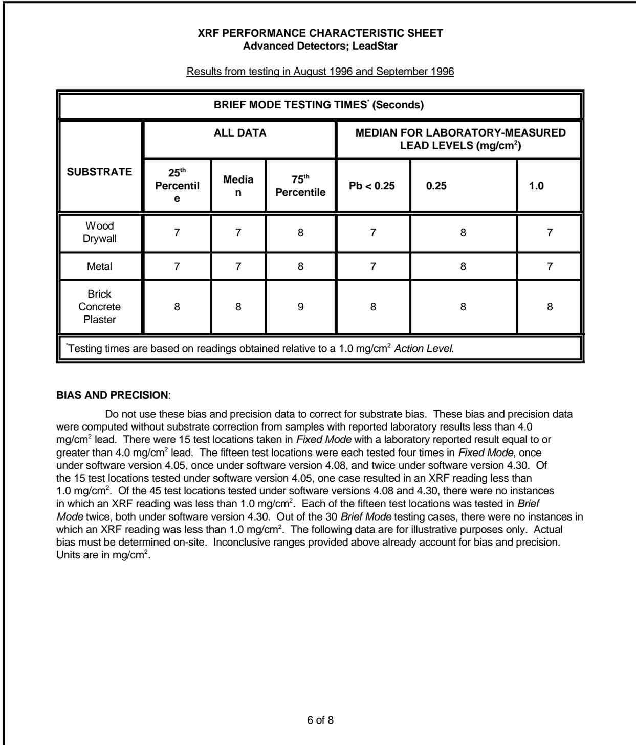
Figure D-1 continued. XRF Performance Characteristic Sheet for the Advanced Detectors LeadStar.
