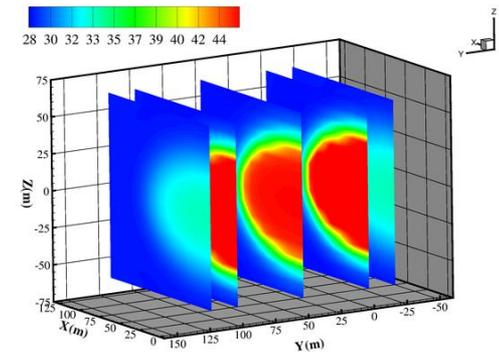
Distribution of pore pressures (MPa) in the formation after 3 hrs of injection
