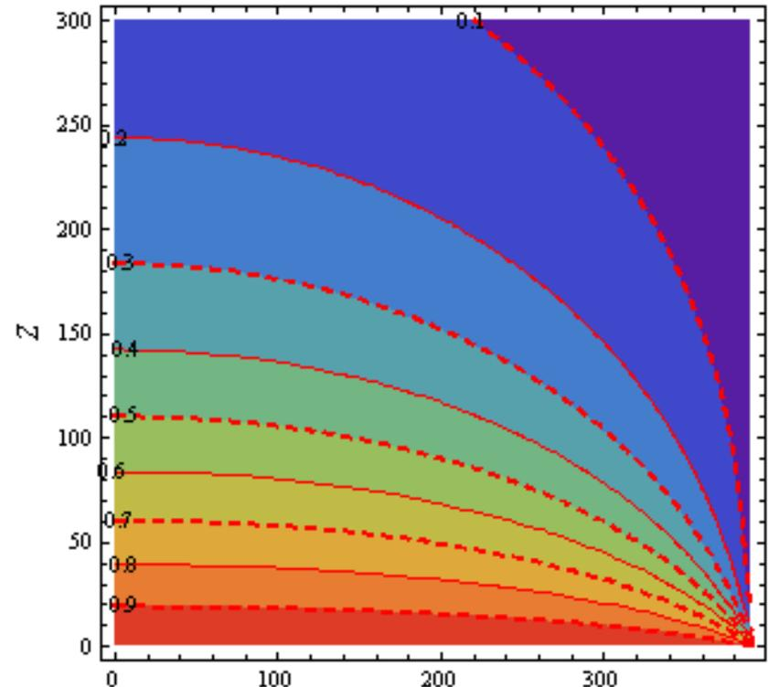
Analytical model for induced stress perpendicular to penny HF (stress shadow)-used for FRV
