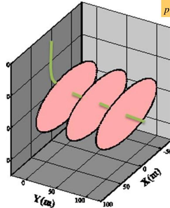
Fracture aperture distribution (in cm) after 3 hours of pumping.
