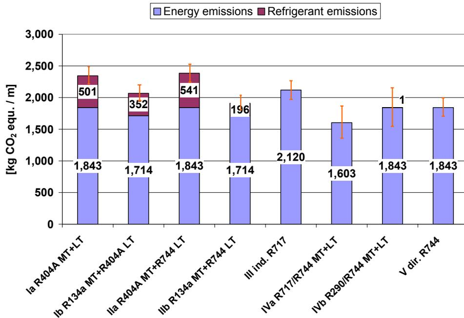
Figure 17: Annual GHG emissions per linear meter of refrigeration unit for the supermarket in connection with different layout options (leakage rate 6.15 %)
