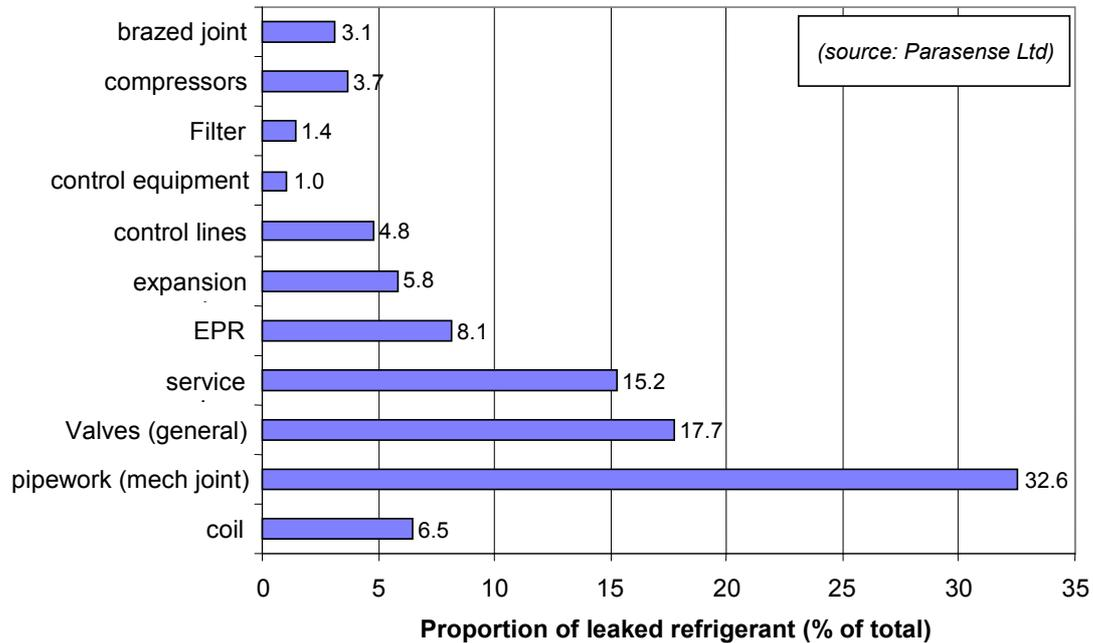
**Figure 17: Refrigerant leakages in central supermarket refrigeration systems in Great Britain [Colbourne2004].**
