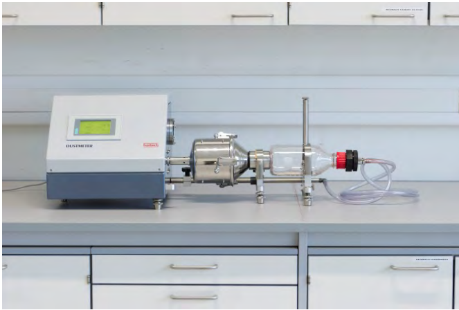
Apparatus with pump, drum and filter case
