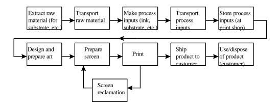
Note: Many more raw materials are used by screen printers than can be indicated in this diagram, which is one reason that making a complete life-cycle process map is very difficult. In addition to ink and substrate, for example, screen printers use screens, stencils, photographic films, film developers and fixers, and screen reclamation solvents.
