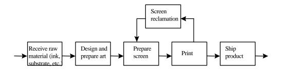
These are the basic processes carried out in a screen printing shop. Of course, many of these processes have separate steps to them. These steps are called unit operations. For example, in some screen printing shops the "screen reclamation" process can be divided into the following separate steps. Different chemicals are applied, and then rinsed off, at each step.
