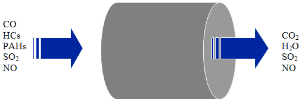
Figure 4-3. Schematic of a Diesel Oxidation Catalyst 9
