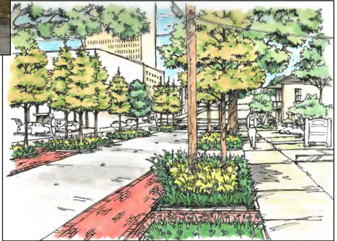
Figure 30. Sketch showing how existing trees could be incorporated into the rain gardens and how on-street parking could be designated with colored paving.
