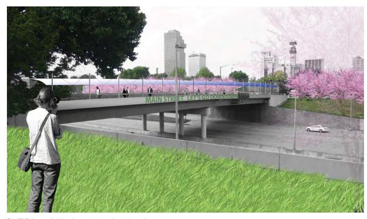
Figure 38: Design concept for bridge enhancements to improve the pedestrian experience.
