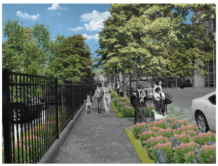
Figure 50: Design concept for a streetscape that includes a streetside rain garden, a parking lane with permeable paving, and a parking lot with a rain garden.
