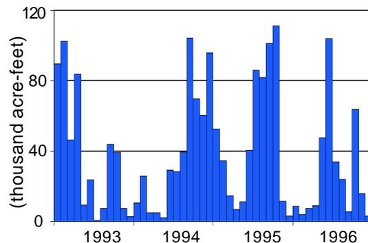
**FIGURE 22.** Monthly discharge at S-8. Discharge varies from zero to several thousand cubic feet per second in response to rain events.
