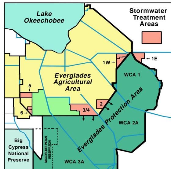
**FIGURE 35.** Location of Phase I phosphorus control program stormwater treatment wetlands. In combination with agricultural best management practices they are to decrease phosphorus to 50 ppb or less prior to discharge into the Everglades (adapted from SFWMD).
