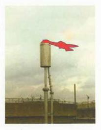
The following image represents a flame below the plane of the exit of the flare tip and attached to the tip. However, since the flame is not discontinuous, this image would not represent Discontinuous Wake Dominated Flow.
