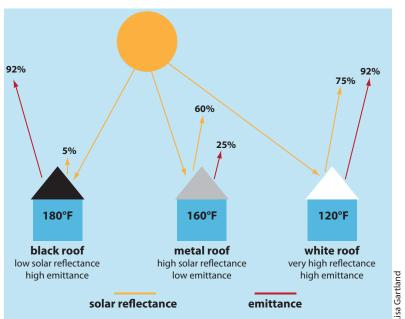
Figure 5: Example of Combined Effects of Solar Reflectance and Thermal Emittance on Roof Surface Temperature<sup>4</sup>
