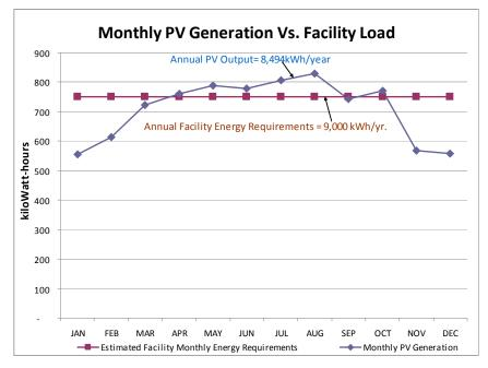
Figure 6-1. Monthly PV Energy Generation Vs. Design Day Facility Energy Requirements
