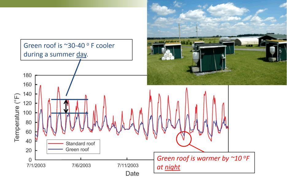
Average rooftop surface temperatures for a standard and a green roof.
