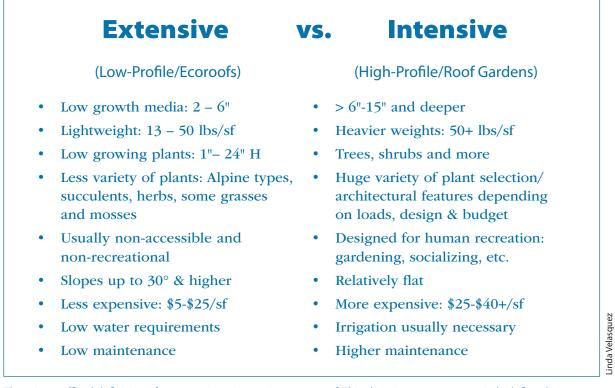
There is no official definition of an extensive or intensive green roof. This chart is not meant to strictly define these green roof types and instead aims to describe the general characteristics of roofs at each end of the continuum.
