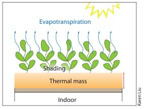
Plant shade reduces the sunlight that reaches the roof. Evapotranspiration further cools a green roof by using heat to evaporate water from the growing medium and plant surfaces
