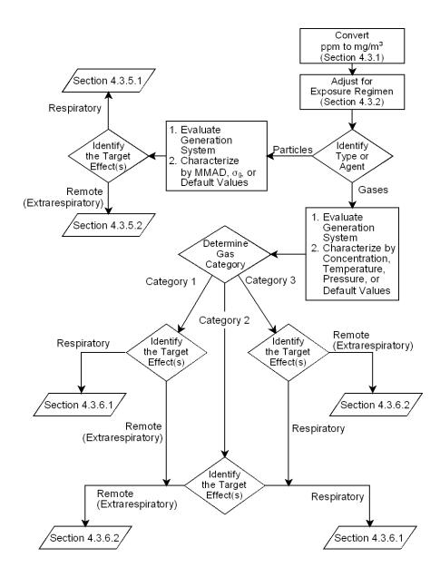
Figure 4-4. Flowchart for calculation of human equivalent concentrations.
