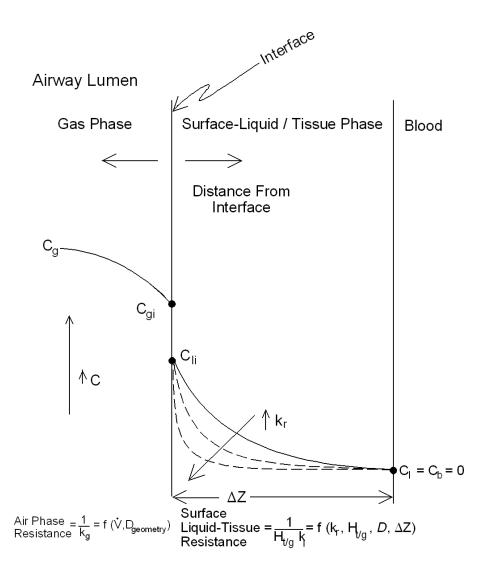
Figure I-2. Schematic of two-phase mass transport resistance model. The definitions for the parameter symbols are provided in Table I-1.
