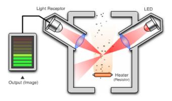
Figure 4. Schematic showing how the particle sensor operates.
