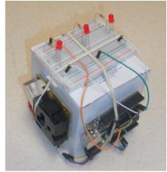
Figure 1. Sensor kit componetns assembled with materials you can find at home (rubber bands, cardboard box)
