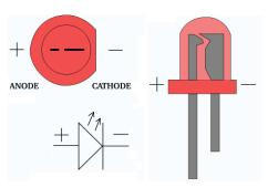
Be aware that an LED is a diode, meaning that it is polarized. By convention, current can only go from the anode (positive end) to the cathode (ground, or negative end)...Note that the two wires on the LED are different lengths. The longer wire is always + and the shorter is -." (Images: http://www.societyofrobots.com/electronics led tutorial.shtml)
