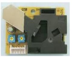
Figure 5. Shinyei particle sensor used in the kit.
