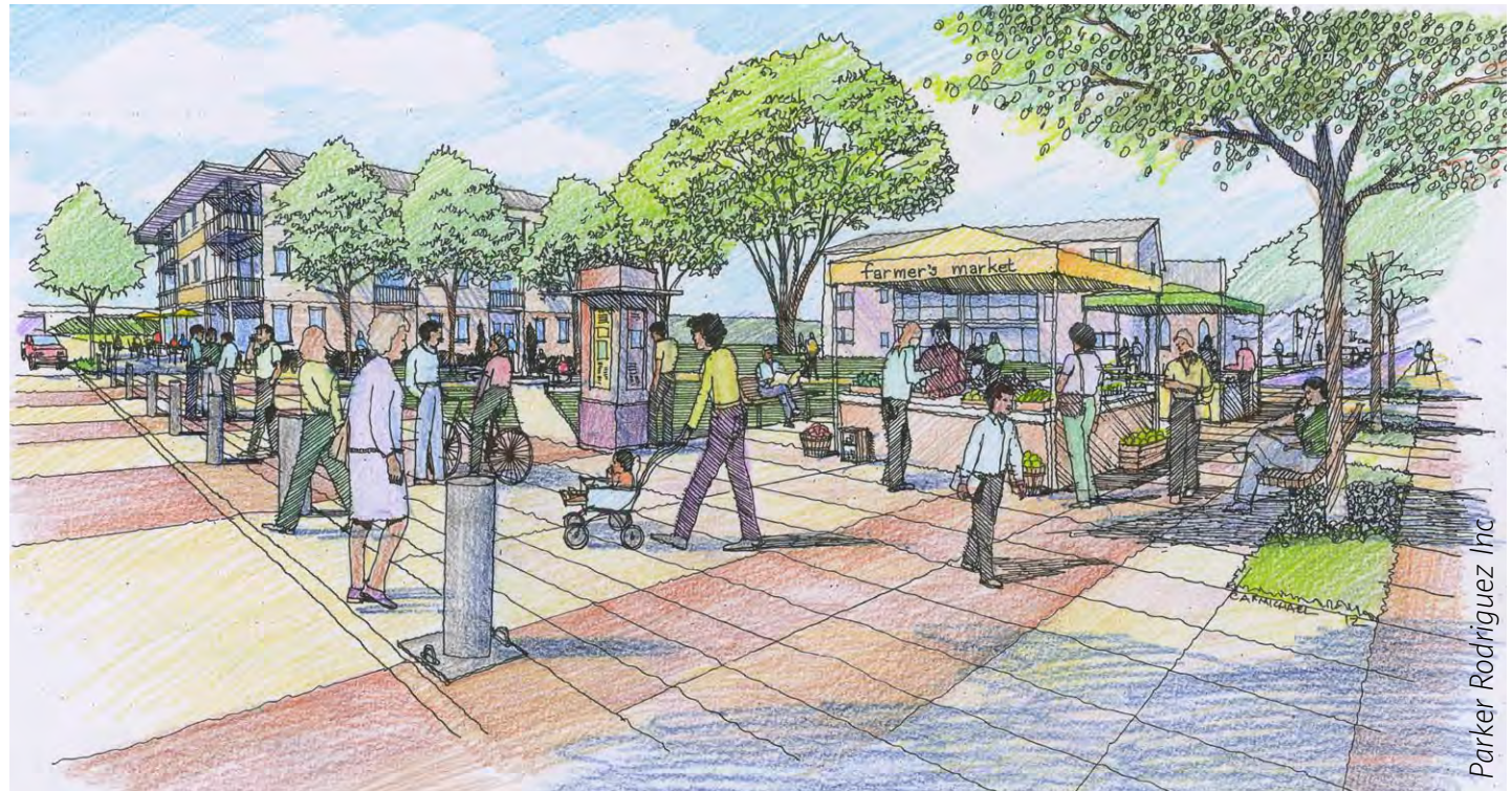
Figure 39: This illustration shows the transformation of Shannon Place from an impervious asphalt cul-de-sac into a place for temporary street festivals. The portion of the existing cul-de-sac remaining as a street would be covered with porous pavement, while the rest of the cul-de-sac would be converted to a landscaped park. Part of the park could be used for a rain garden to capture and filter stormwater on the site (see Appendix C). Existing trees in the area would remain. The illustration shows the potential for new infill development that matches the scale and character of the existing building. The plaza could be used for neighborhood events such as a farmers market, which could provide locally sourced food to the community. A kiosk could provide wayfinding information and serve as a community bulletin board.
