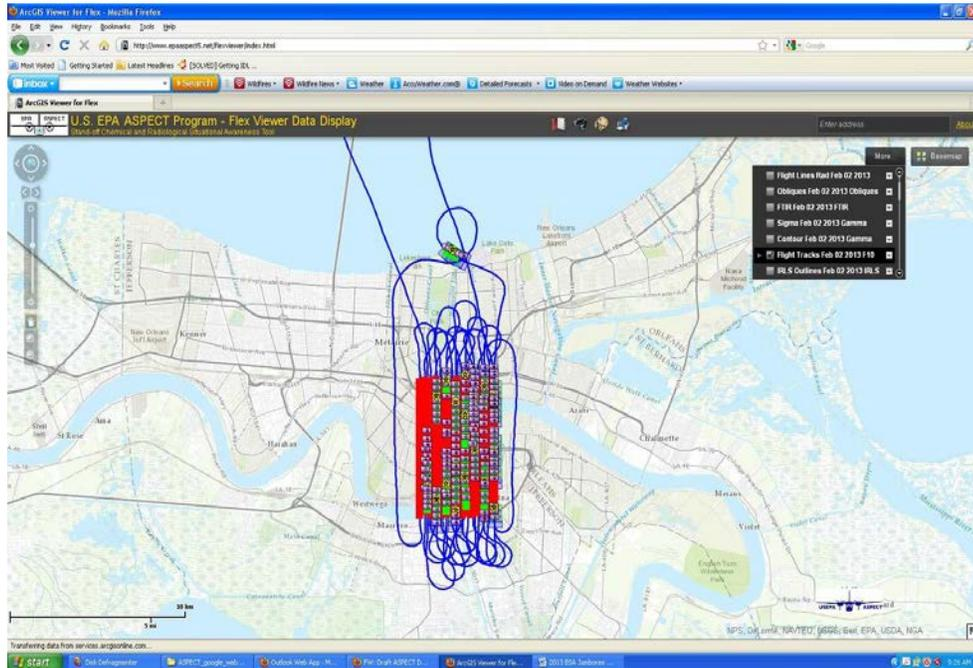
Figure 18. Sample ESRI Flex Viewer Display of ASPECT Aircraft Tracks. The red tracks indicate when radiological sensors were actively taking measurements.
