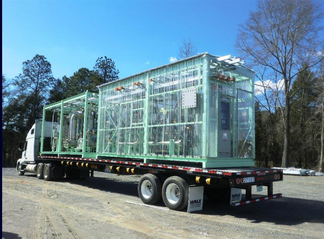
Assembled in 20ft. Standard Conex Frames
