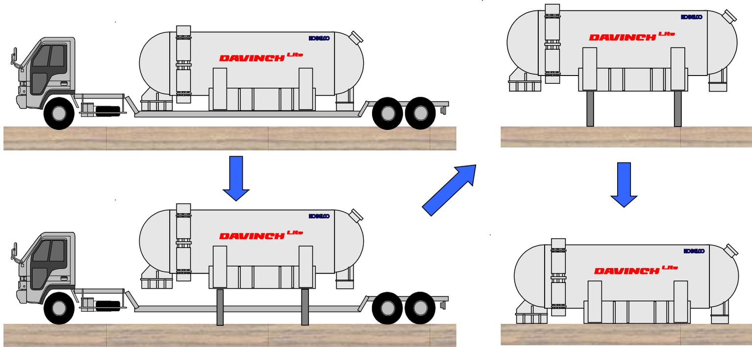
No crane is required for installation
