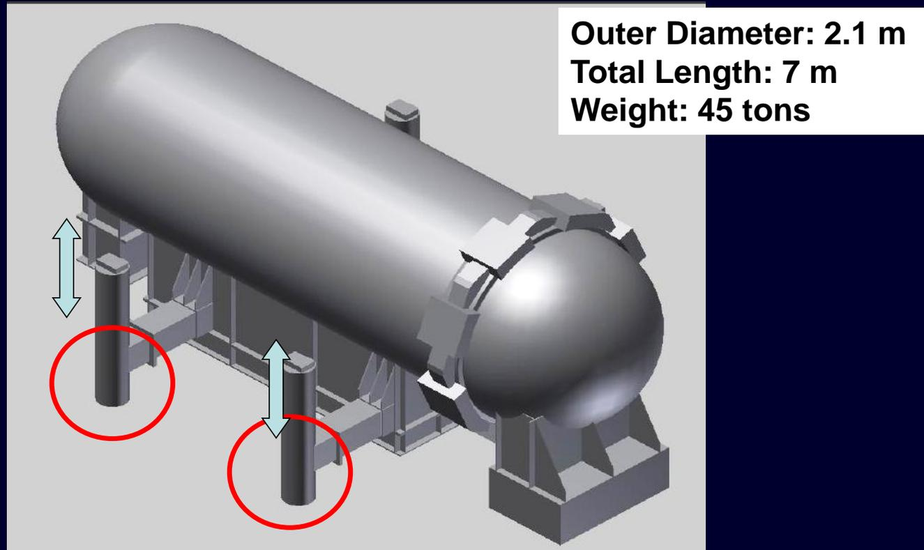
Self Unloading System by Outrigger
