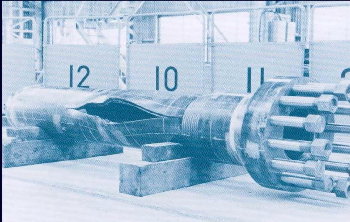
Example of Burst-Before-Leak,
