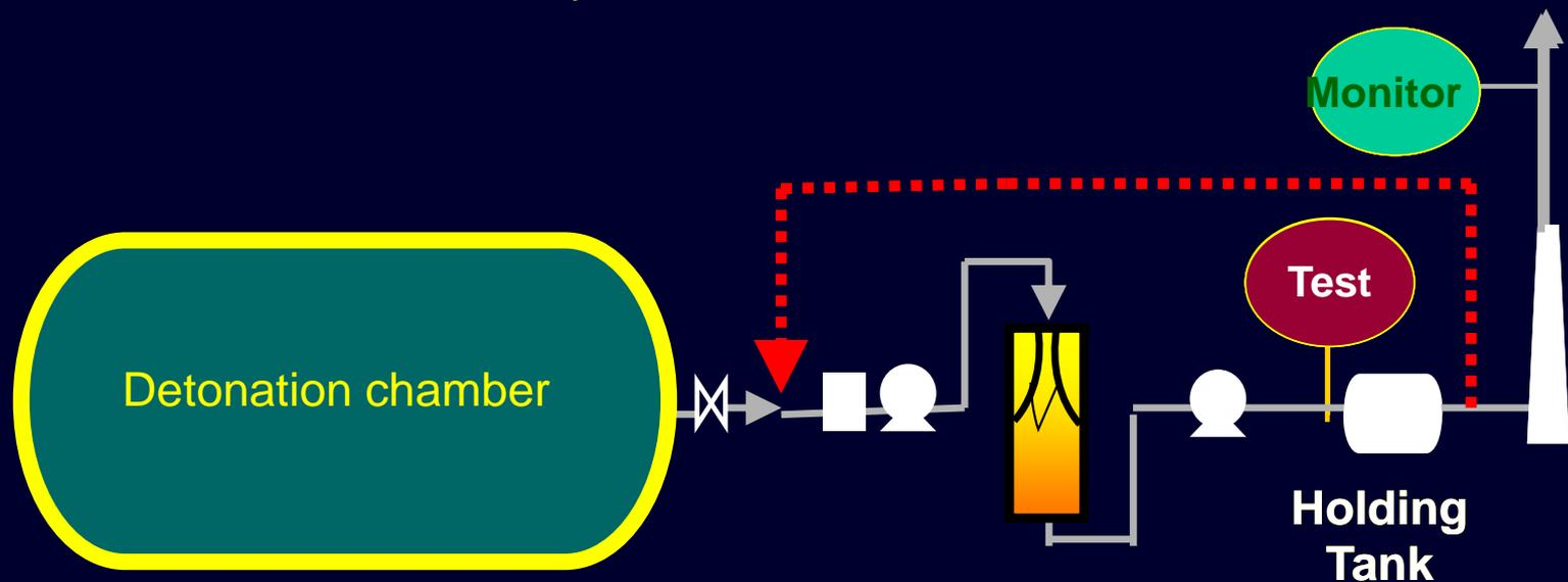
*All off gases are compressed and held for analysis. Non-compliant batches are recycled until clean.*
