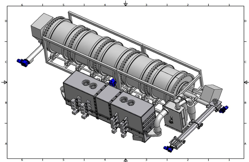
Fig.3. HR 5000 and block of MOS reactors.
