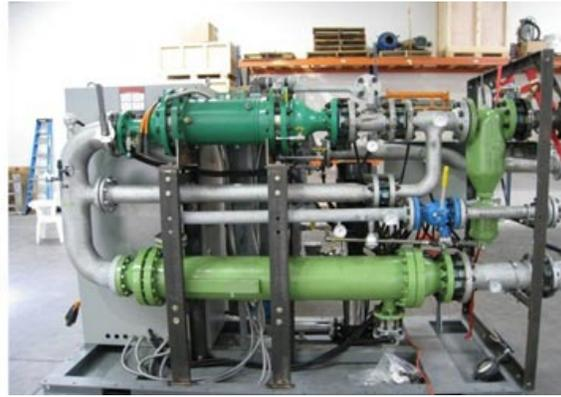
Fig. 6. ORC system for electricity generation
