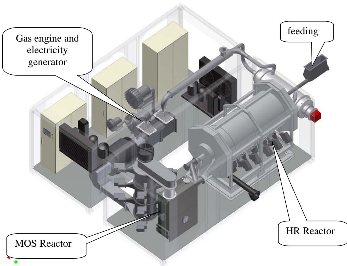
Fig.2. Complete system with HR 200 and MOS reactors.
