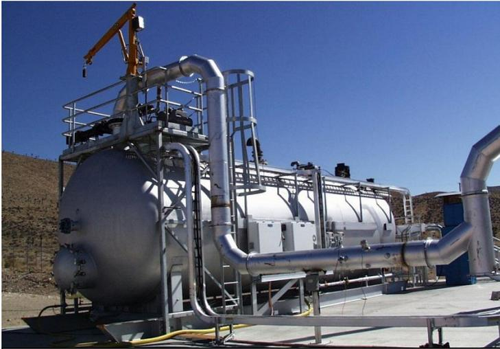
**Figure 3. Pressure vessel designed to dispose of Shillelagh missiles.**
