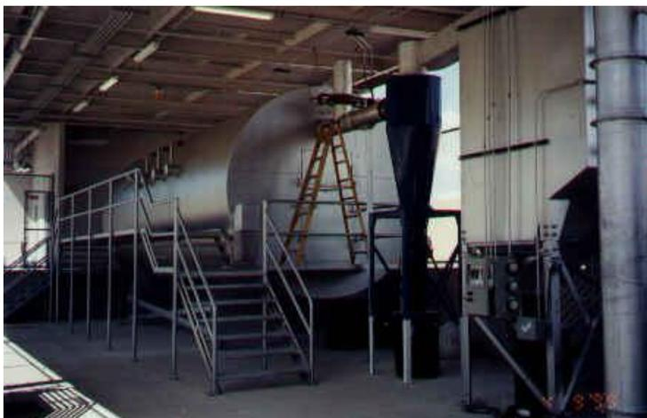
**Figure 2. Semi-continuous system uses solid fuel as ignition source for wastes**
