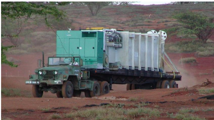
**Figure 3: Transportable Flashing Furnace**
