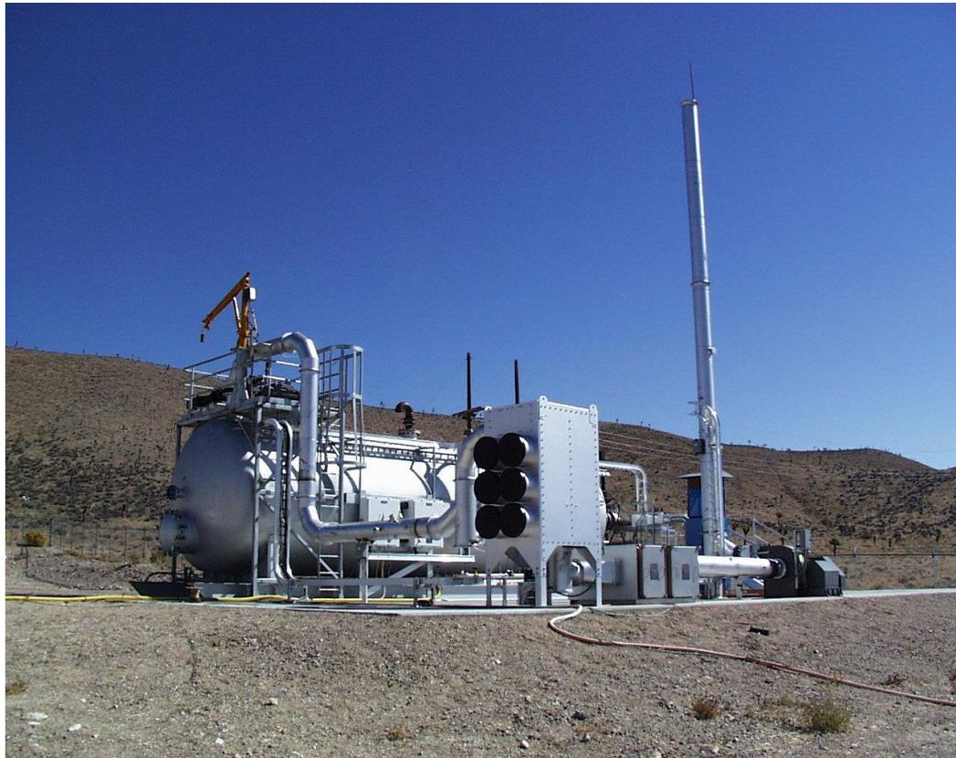
**Nitrocellulose Based Propellant Contained Burn System
