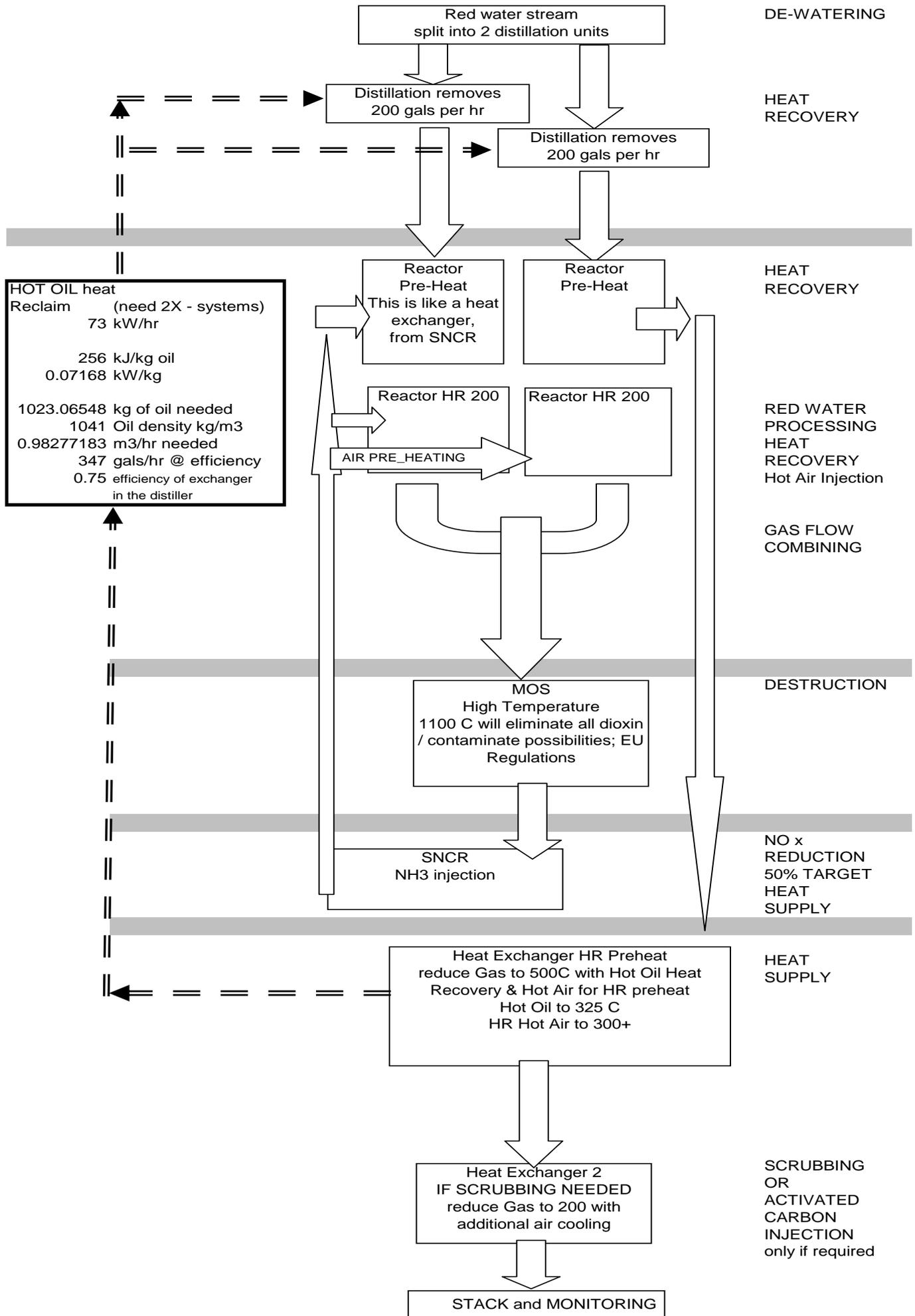
**FLOW BALANCES : Follows is a proposed operation mass flow. Any additional de-watering of the waste stream at the vacuum distillation (VD) step is a benefit to the entire process.**
