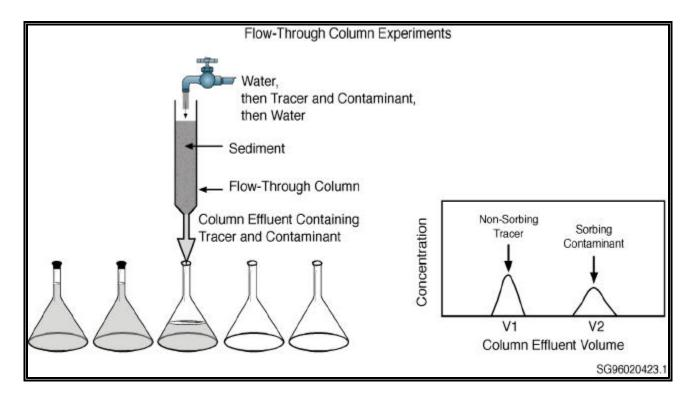
**Figure 3.3**. Procedure for measuring a column  $K_d$  value.
