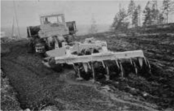
Incorporation of high rates of biosolids mixtures similarly requires the proper equipment and equipment operators. The low % solids of the biosolids means that when you are making a 100 dry t/ac application, you may actually be applying over 500 wet t/ac of material. Generally a large track bulldozer (such as a Caterpillar D7) pulling a 36" disk is required. Smaller equipment will just float on the surface of the biosolids mixture. Large chisel plows also exist that are capable of inc
