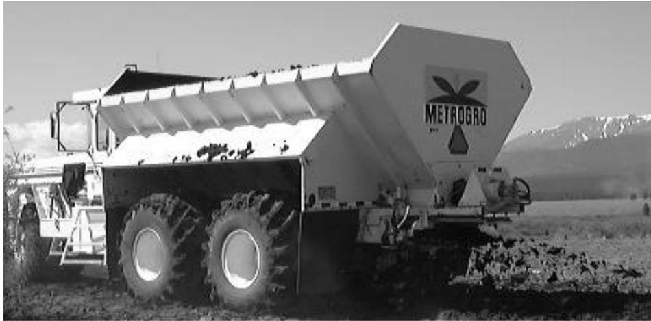
They spread biosolids from the rear of the box with a fan or splash plate. The width of the spread is comparable to the width of the vehicle. Changing the speed of the vehicle as well as the speed of the fan can alter application rates. These vehicles are excellent for
