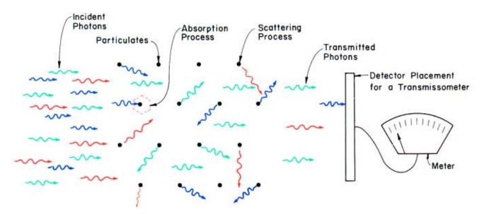
Fig. 5.2 Placement of a light source and detector as shown here is known as a transmissometer. As photons pass through a concentration of particles and gases, they are either scattered out of the light path or they are absorbed. Thus a detector placed as indicated measures only those photons that are transmitted the length of the light path. Because this instrument is sensitive to both scattering and absorption, it can be calibrated to measure the extinction coefficient.
