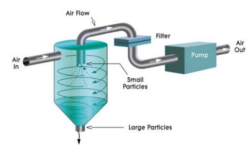
Fig. 5.4 Diagram of a cyclone-type particle monitor. The air inside the cyclone spins in such a way as to cause larger particles to deposit on the inside of the monitor and fall to the bottom, while smaller particles continue in the air stream and are collected on a filter substrate for analysis.
