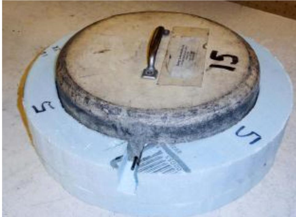
The Large Area Activated Charcoal Canisters (LAACCs) fit snugly in the float to create a seal.
