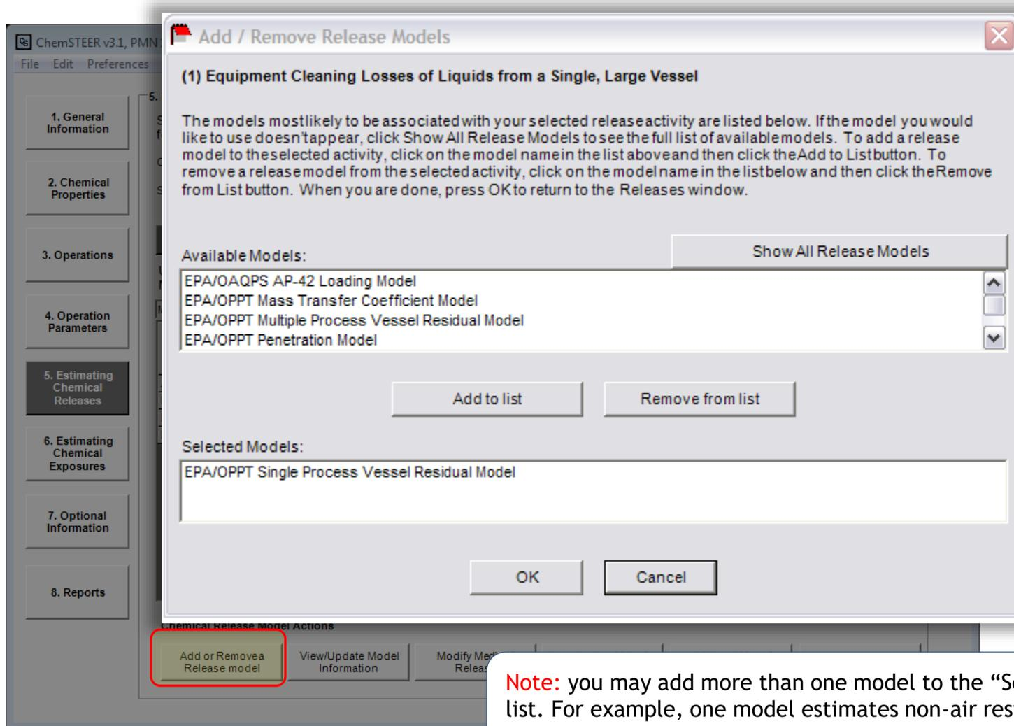
The upper window shows the most appropriate alternative / additional models for the selected release source.
