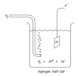
If, as shown in Figure 2, a SHE is connected with a salt bridge to a second half-cell in which a reduction reaction is taking place, the electric potential between the two cells can be measured. In the case shown, the potential of the right cell will be +0.34 Volts in reference to the standard hydrogen electrode on the left. This would be represented as an Oxidation Reduction Potential (ORP) of +340mV on the hydrogen scale, or simply as Eh = +340mV.
