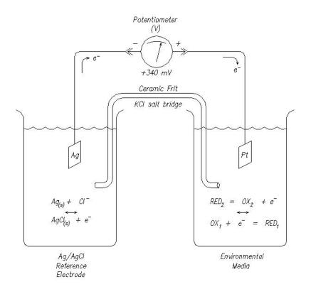
In this illustration, the ORP is measured as 340 mV. This measurement is made in reference to the Ag/AgCl reference electrode and would be reported as such, or as  $E_{Ag/AgCl} = 340$ mV.
