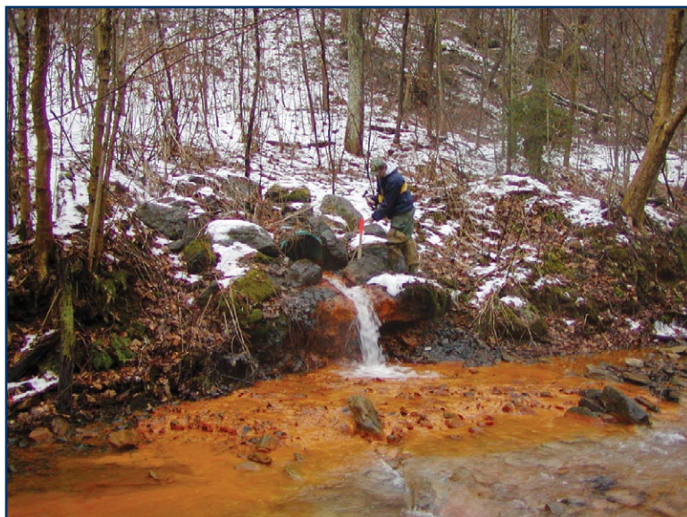
Acid mine drainage flows into Possum Hollow, a Morris Creek tributary, West Virginia.
