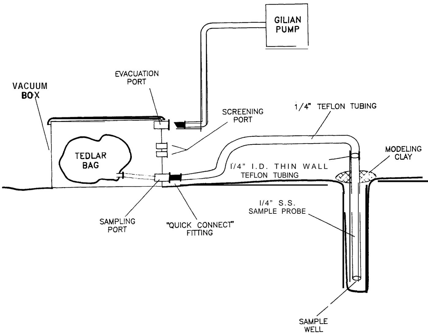
Figure 1: Sampling Train Schematic
