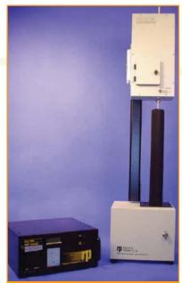
The Series 8500 FDMS<sup>™</sup> unit has been selected by the California Air Resources Board as a California Approved Sampler for both PM<sub>2.5</sub> and PM<sub>10</sub>.
