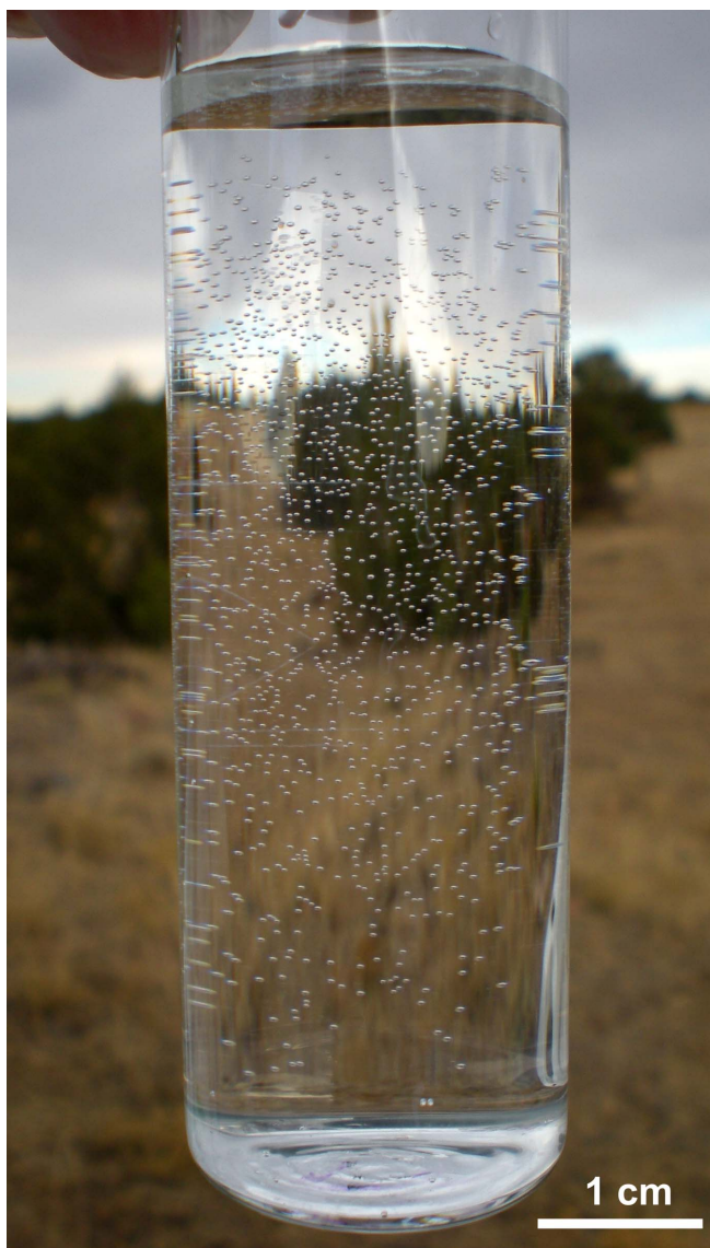
Figure 36. Gas exsolution in ground water collected from domestic well RBDW09, located within the Little Creek Field study area (Huerfano County), during the November 2012 sampling event. The bubbles reflect a mixture of dissolved gases: results from headspace gas analyses (Appendix B, Table B-8) indicated the presence of methane (44.3%), nitrogen (54.3%), argon (0.99%), carbon dioxide (0.31%), and ethane (0.03%). (Vial diameter = 2.4 cm).
