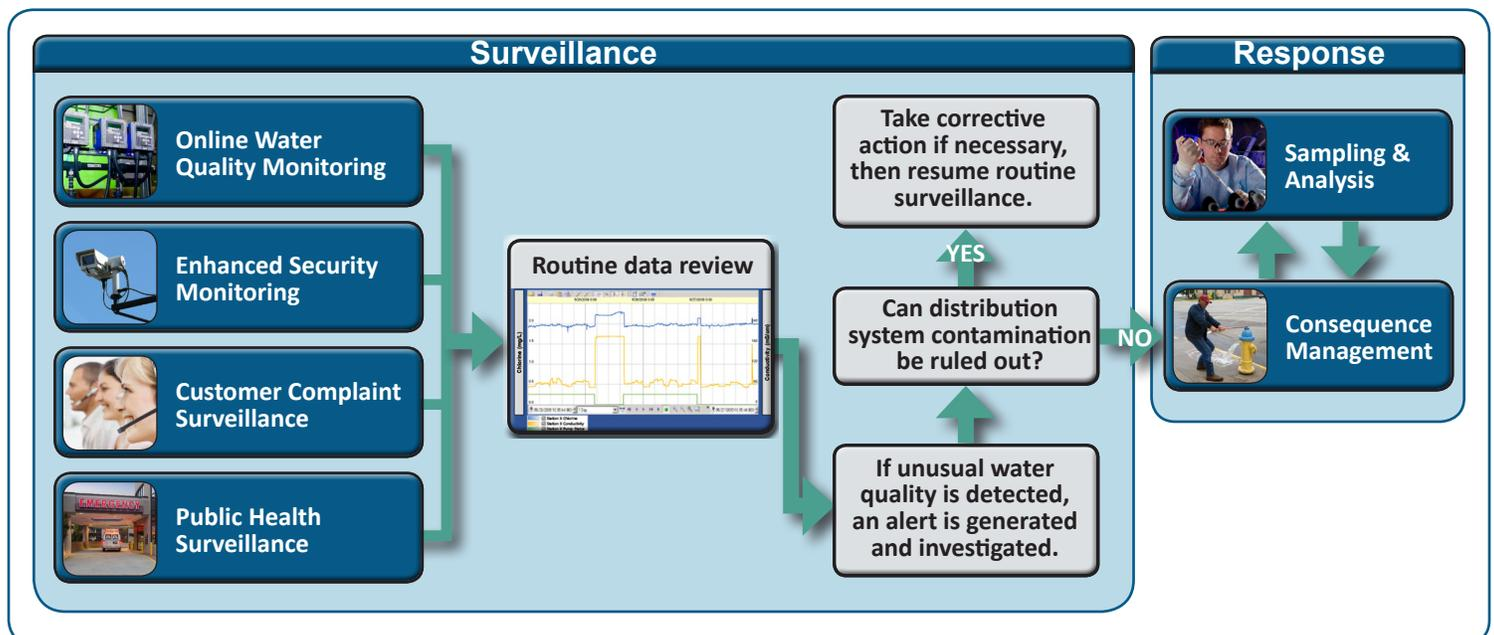
**Online Water Quality Monitoring** involves continuous monitoring of water quality parameters at strategic locations in the distribution system. Data from these monitoring stations is automatically transmitted to a central information management system and analyzed to detect unusual water quality conditions. Measured water quality parameters include:
