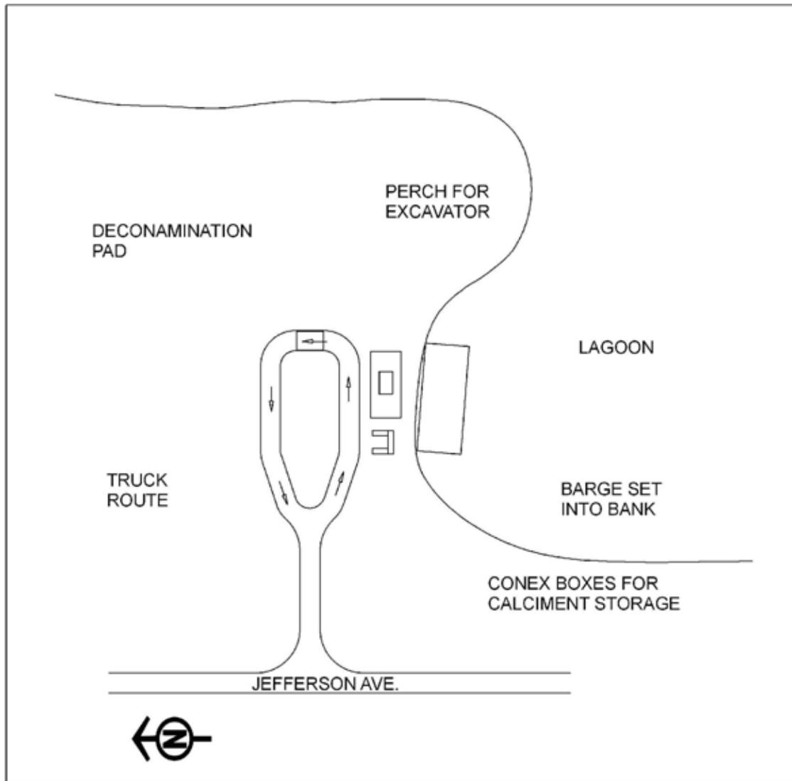
Figure 4-2 Schematic Drawing of Contingency Trucking Operations
