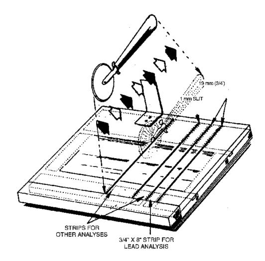
Figure 2. Diagram of filter cutting procedure.
