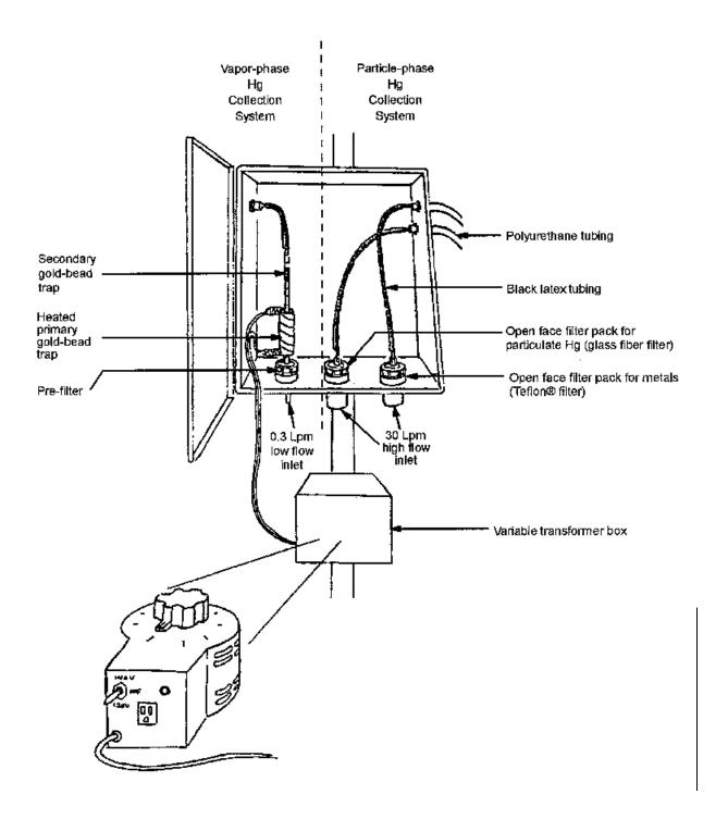
Figure 1. Example of ambient sampling system for collection of vapor and particle phase mercury.
