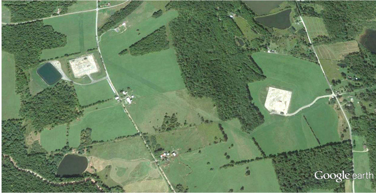
Figure 4-8. Aerial view of terrain, land use, and well pads in Bradford County. Distance between the two well pads is about 3500 feet. Multiple hydraulic fracturing wells can be drilled from one pad. The well pad in the upper left corner has a fracturing-operator-constructed freshwater storage pond. (Image Google Earth, PADCNR-PAMAP/USGS.)
